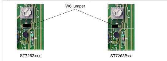
Figure 2. Device selection for analog-to-digital conversion
