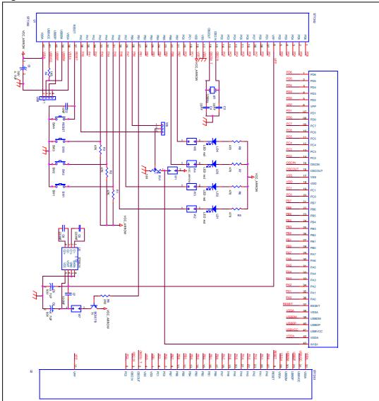
Figure 6. Board schematics
